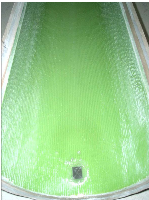
Figure 15: Sample item B1003-1.1 after the abrasion test with 200,000 load alternations
