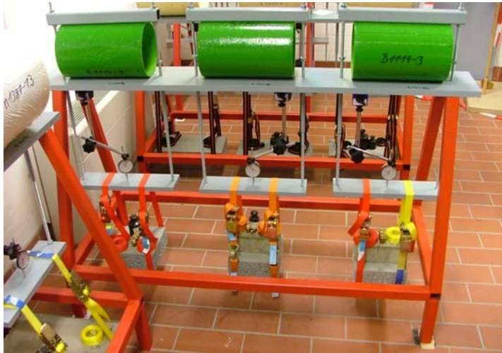
Fig. 17: Test station for the long-term peak compressive test in the IKT.
